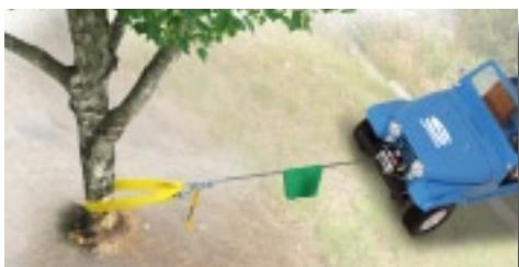
A typical double-line winch and pulley arrangement doubles winch capacity.
