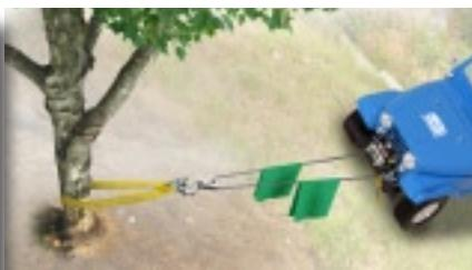
A redirected pull. If there's no straight, clear line to the anchor point, use a pulley block.
